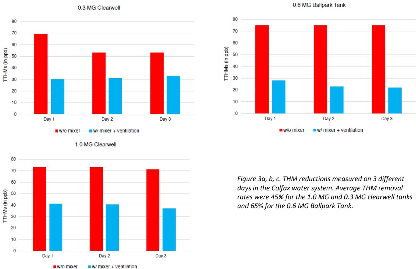
Figure 3a, b, c. THM reductions measured on 3 different days in the Colfax water system. Average THM removal rates were 45% for the 1.0 MG and 0.3 MG clearwell tanks and 65% for the 0.6 MG Ballpark Tank.
